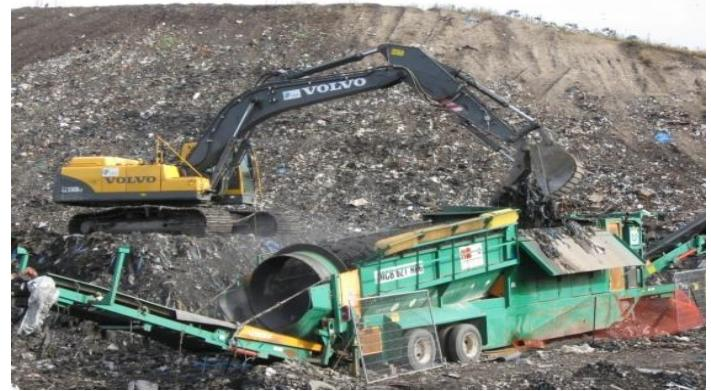
Figure 1. Photographs showing the landfill soil reclamation process: material post screening (left) and screening plant (right).
