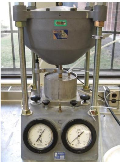
Figure 4. Sample cell seated in pneumatic consolidation cell.
