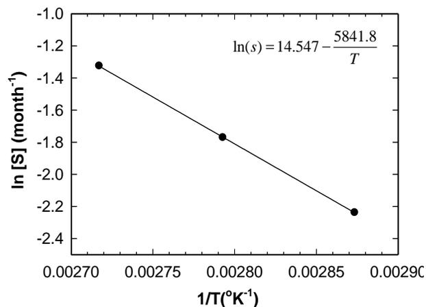
Figure 3. Arrhenius Plot of the antioxidant depletion for GMB<sub>1</sub> immersed in Solution 1 (Table 1)
