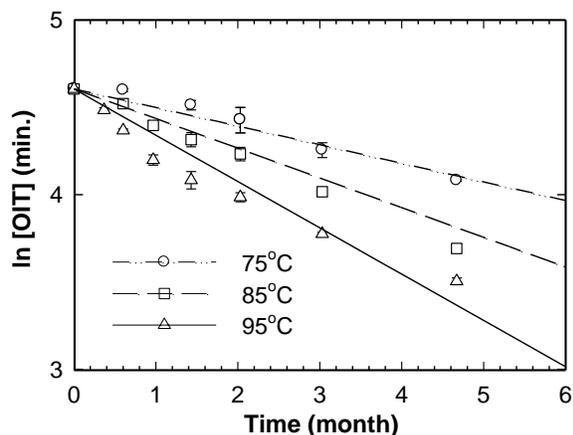
Figure 2. Antioxidant depletion rates (Std-OIT) for GMB<sub>1</sub> in solution 1 at three temperatures
