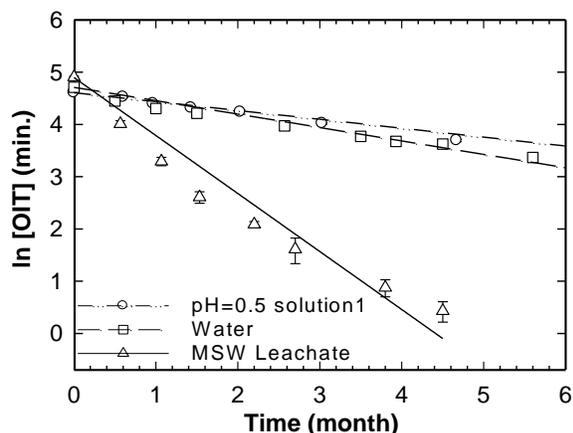
Figure 4. Std-OIT depletion for GMB<sub>1</sub> in different immersion fluids at 85°C (water data from Rowe et al. 2010a and MSW leachate data from Rowe et al. 2010b).
