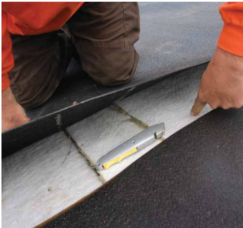
Figure 8 | Photos showing location on long slope where GCL was exhumed, and the exhumed seam (orange dots in middle of slope are people cutting the geomembrane). GCL was observed to be hydrated, and the heat-tacked seam was intact.
