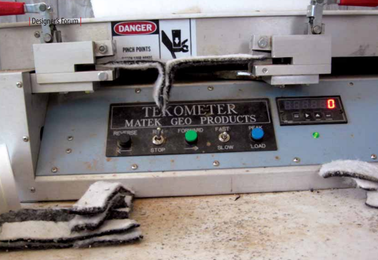
Figure 9 | Performing shear and peel tests on 1-in. wide strips of heat-bonded GCL seams.
