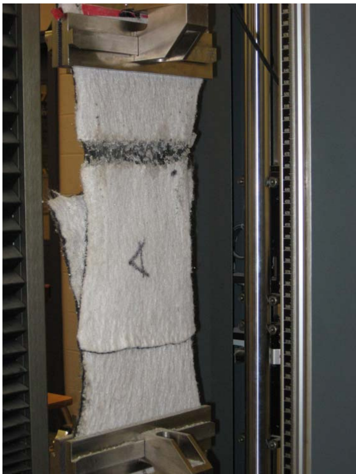
Figure 9. Tensile failure of specimen by pre-engineered groove.
