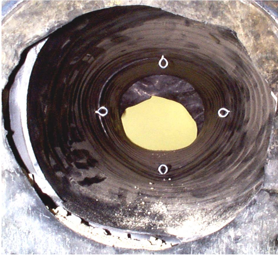
Photo 5: PE Drain Pipe After 2,000 kPa Loading
