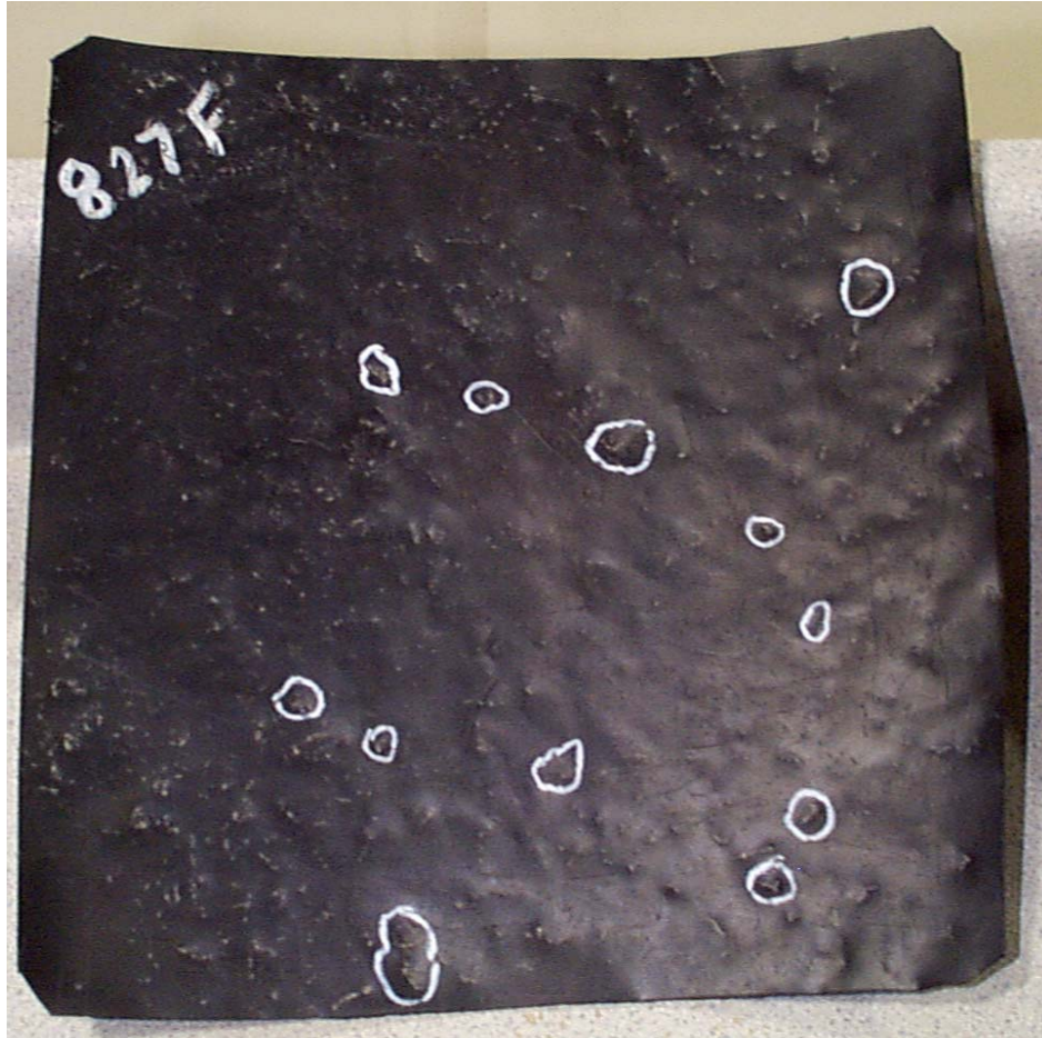
Photo note: White circles mark locations of incipient failure.
