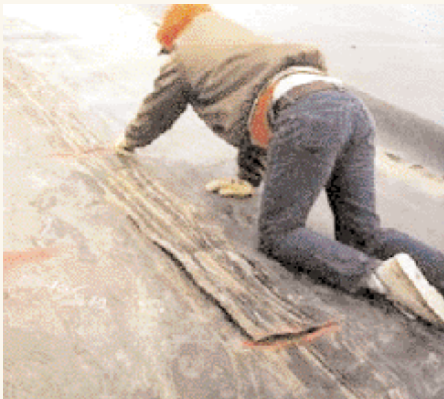
Photo 1. Cutting holes in geomembrane for testing.
