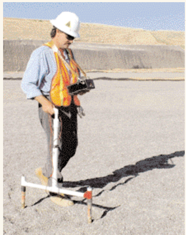
Photo 2. Testing geomembrane for holes and cuts.
