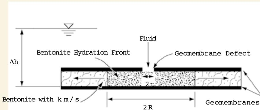
Figure 2: Drawing illustrating factors for calculating radial hydration of encapsulated bentonite through a geomembrane defect.
